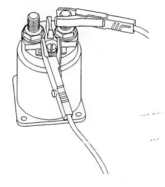
COMPONENT CHECKING AND REPAIR Checking solenoid switch Use tester to check resistance of holding winding (term. 50/ground). Alternator tester: 0 684 201 200 Holding winding resistance Starting motor - 0 001 223 0..: 1,1...1,3 Ohm Starting motor - 0 001 223 5..: 1,0...1,1 Ohm
